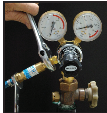
Figure 3. Attaching Fuel Gas Regulator.
