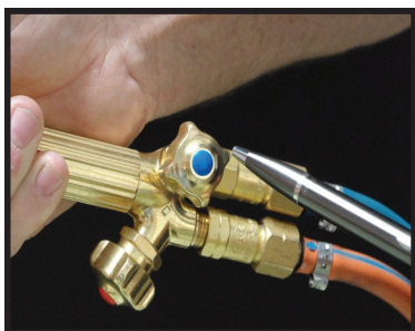
Figure 14. Open valves & Purge gas
