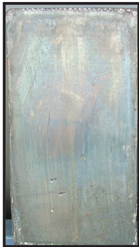
Figure 19. Steel Flame Cutting
