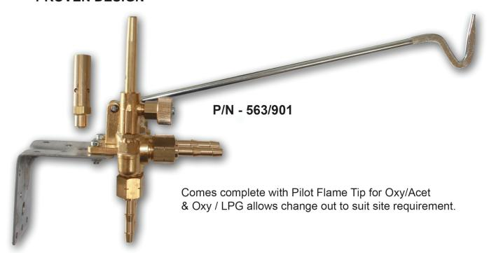
Automatic interruption of gas supply by placing the torch on the hook - no readjustment of settings necessary when unhooking the torch. Adjustable pilot flame - available for oxygen-acetylene, propane/natural gas. Detachable 6 mm hose nut and nipples to suit gases.
